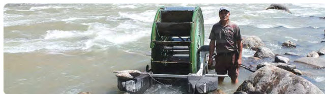
A river-current pump lifting water with no fuel or grid power
